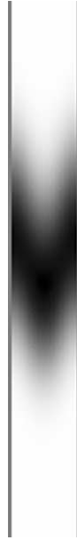
Fig. 10. Two-dimensional simulation of Taylor–Aris dispersion, steady-state flow and transport between parallel plates. Gray scale denotes concentration distribution with black corresponding to maximum concentration and white to the zero solute concentration.
